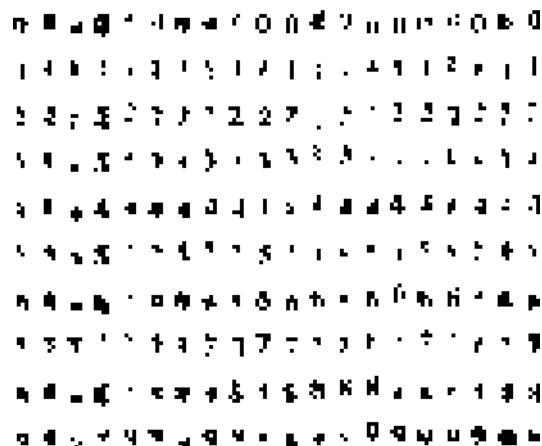
Figure 3: Twenty images each of the ten Times Roman digits 0-9 (top to bottom), generated pseudo-randomly at a type size of 5 point and a spatial sampling rate of 100 pixels/inch. We have shown that, in spite of the extreme distortions, this problem has an intrinsic error rate of only 35%.
